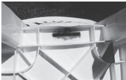
Mold growing on the underside of a plastic lawn chair in an area where rainwater drips through and deposits organic material.
